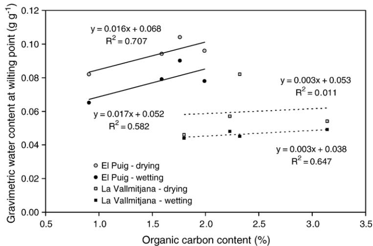
Fig. 8. Relationship between mean gravimetric water content at wilting point ( $\psi = 1.5$  MPa) and mean organic carbon content for the different sludge treatments on the two soils. Drying and wetting refer to the main drying and wetting branches for the water retention curve, respectively.
