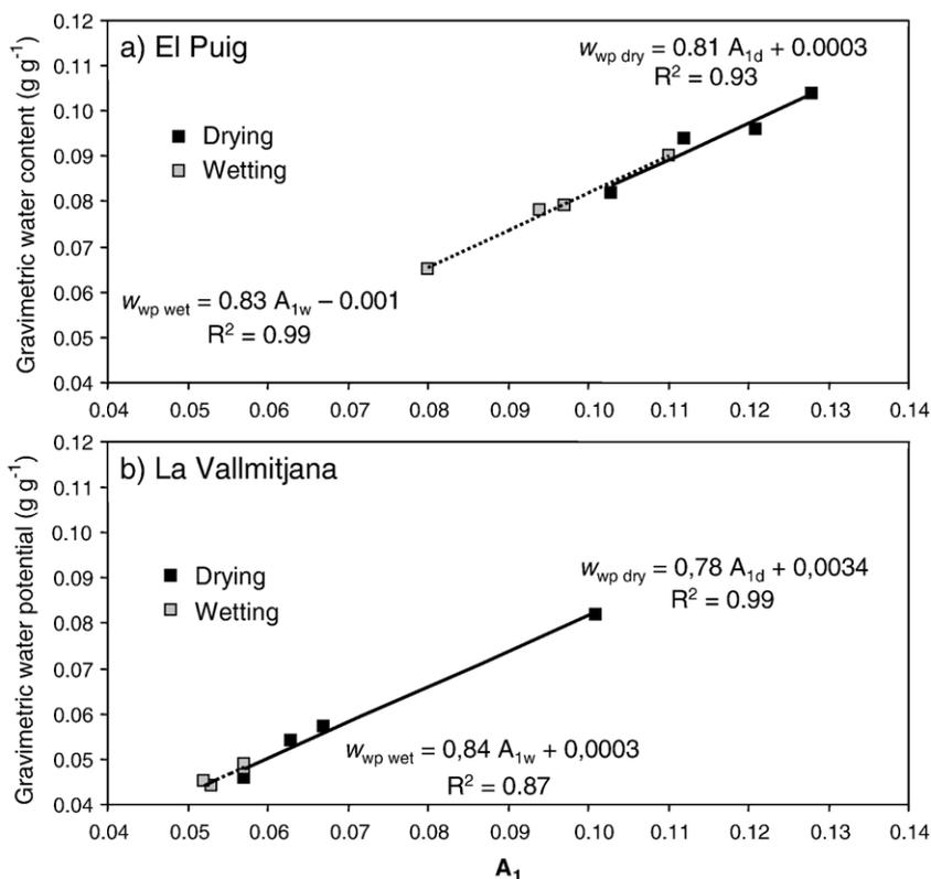
Fig. 7. Relationships between mean gravimetric water content at wilting point ( $\psi=1.5$  MPa) and the  $A_1$  parameter for the different sludge treatments on the two soils. Drying and wetting refer to the main drying and wetting branches for the water retention curve, respectively.
