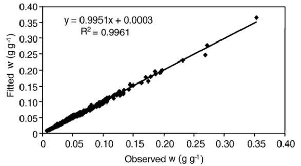
Fig. 1. Fitted gravimetric water contents from best fits of Eqs. (12a)/(12b) vs. observed values for both soils ( $n=667$ ).
