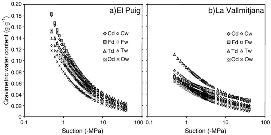
Fig. 3. Mean fitted water retention curves for all treatments (O=control; C=composted sludge; F=fresh sludge; T=thermally dried sludge), in both states (w: wetting; d: drying) and both soils.
