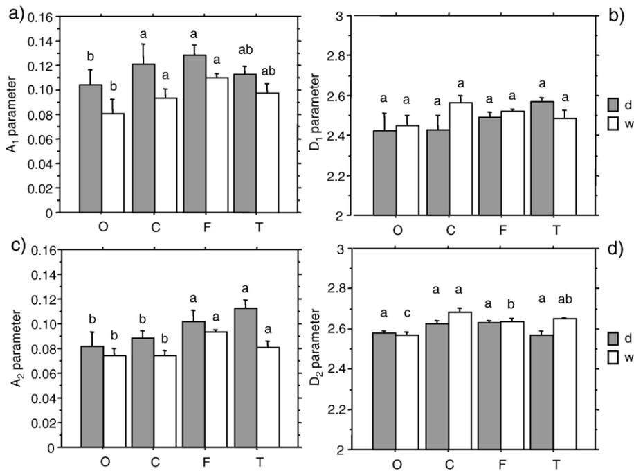
Fig. 4. Mean values of (a)  $A_1$ , (b)  $D_1$ , (c)  $A_2$ , and (d)  $D_2$  for the different sludge treatments (O=control; C=composted sludge; F=fresh sludge; T=thermally dried sludge), in both states (w: wetting; d: drying) on the El Puig loam soil. Bars with the same letter are not significantly different at  $p < 0.05$ .
