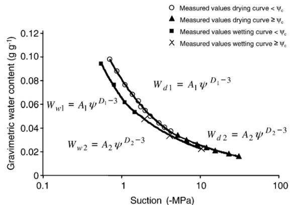
Fig. 2. Example of the segmented fractal model used to fit the main drying and wetting branches of the water retention curve applied to a sample from the loam soil (subscript d: drying state; w: wetting state;  $\psi_c$ : critical matrix potential).
