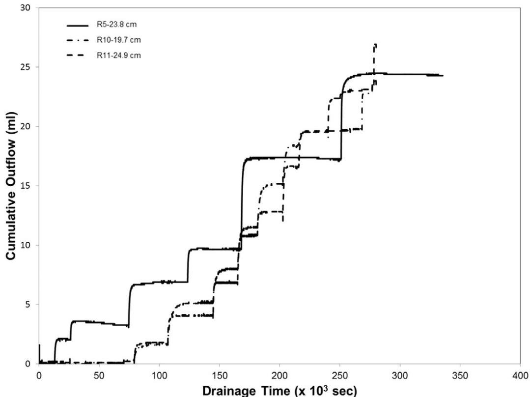
Fig. 2. Cumulative water outflow through time for the 23.8 cm, 19.7 cm, and 24.9 cm Flint sand hanging water column drainage experiments.
