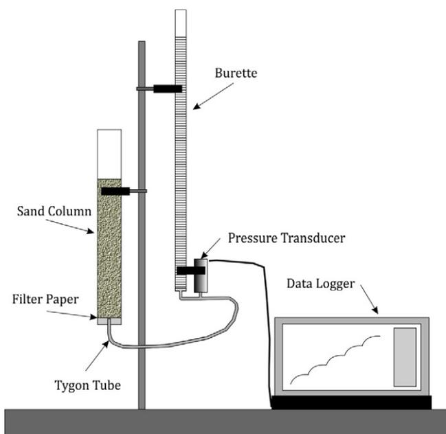
Fig. 1. Hanging water column laboratory setup showing sand column, burette, pressure transducer, and data logging computer.
