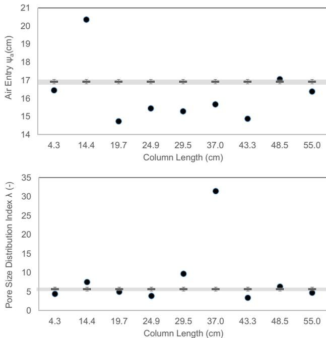
**Fig. 4.** Relationship between TrueCell (Jalbert et al., 1999) estimates of air entry ( $\psi_a$ ) parameters and pore size distribution index ( $\lambda$ ) parameters shown as circles, and parameter values determined by neutron imaging. Neutron imaging values are shown as dashes with 95% confidence intervals as error bars (gray).
