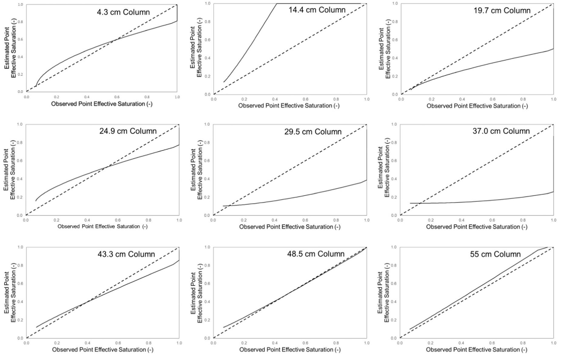
**Fig. 5.** Estimated point effective saturations determined using parameter sets from TrueCell for nine column heights of Flint sand compared with observed point effective saturations determined from the parameter set obtained by neutron radiography. The dashed line indicates one to one correspondence.
