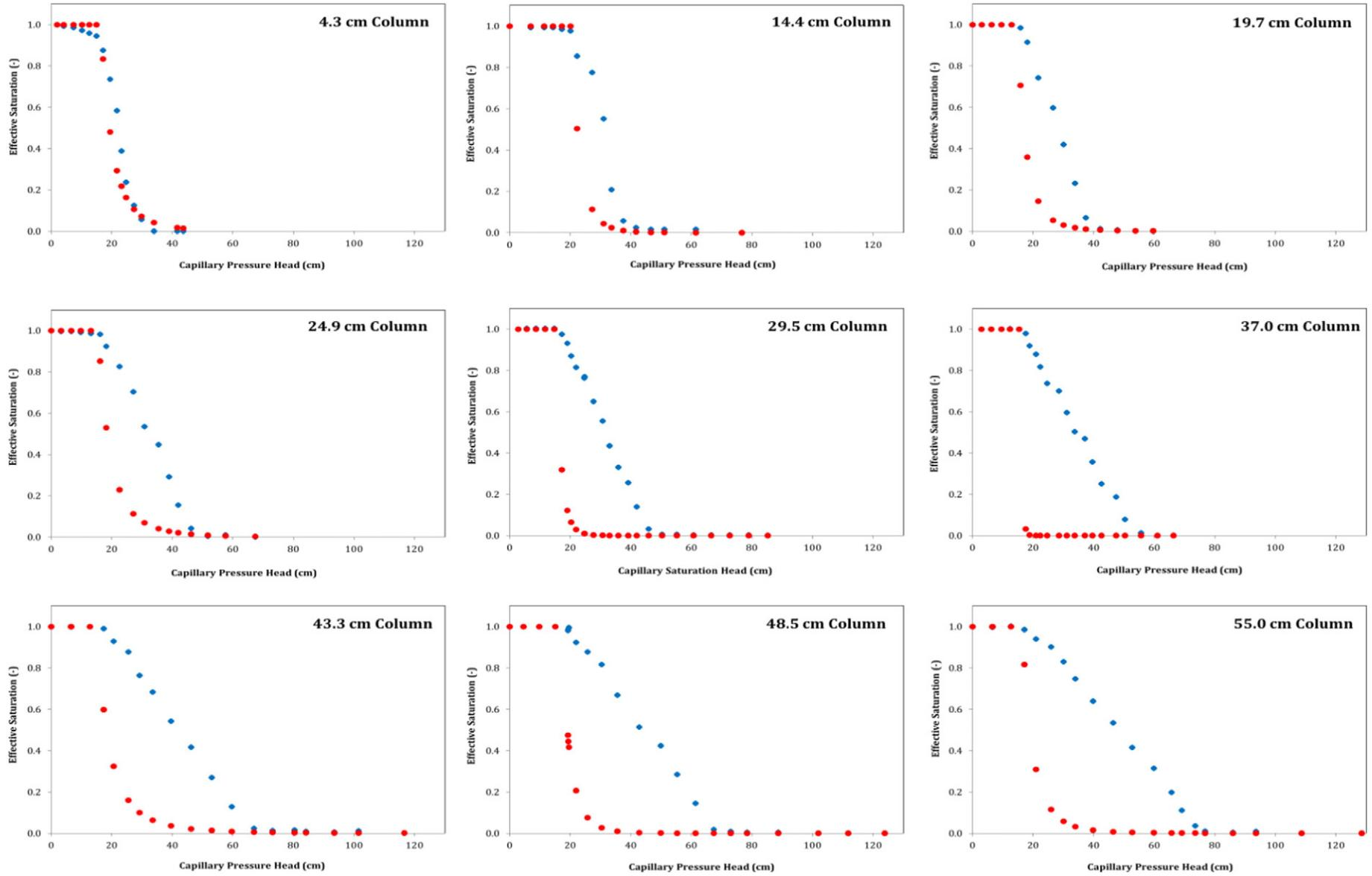
Fig. 3. Measured average capillary pressure–effective saturation data pairs (blue) and predicted point values (red) from TrueCell (Jalbert et al., 1999) for the nine column heights of Flint sand.
