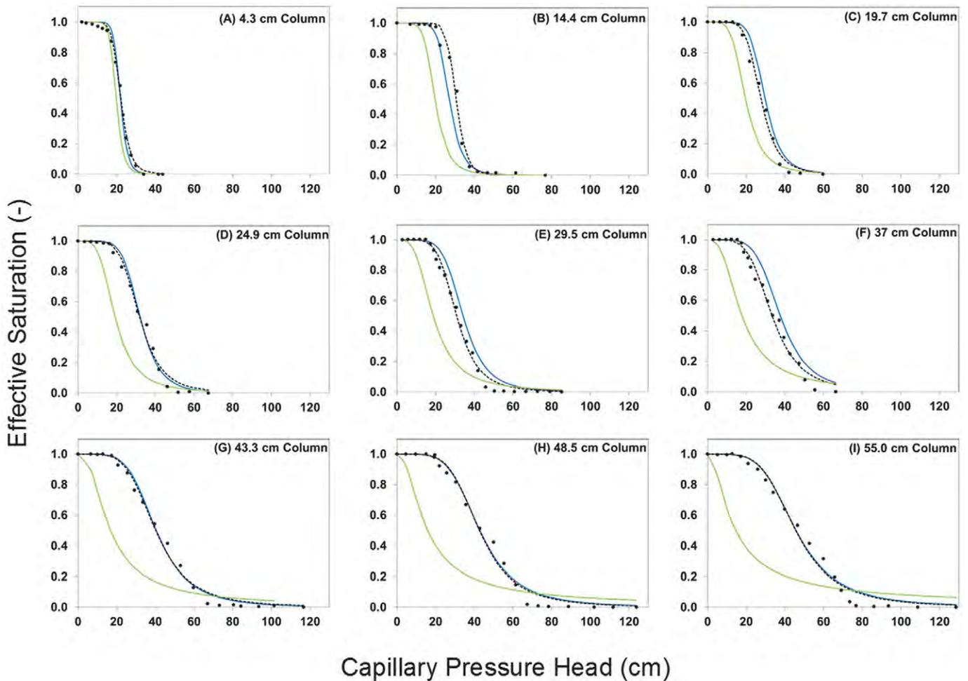
Fig. 4. Upscaled top (solid blue lines) and midpoint (solid green lines) reference pressure elevation predictions of capillary pressure–effective saturation functions compared with measured average data points (black circles) and van Genuchten (1980) functions fitted to measured average data points (dashed black lines) for Flint sand packed into nine columns with different heights ranging from (A) 4.3 cm through (I) 55.0 cm.
