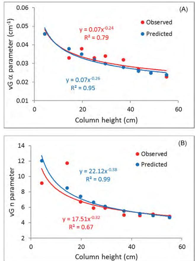
Fig. 5. Column height dependencies of the (A)  $\alpha$  and (B)  $n$  parameters in the van Genuchten (1980) effective saturation–capillary pressure head equation predicted by the BC-vG Upscaler and fitted to the observed average drainage data. In both cases, a top reference pressure elevation was used.
