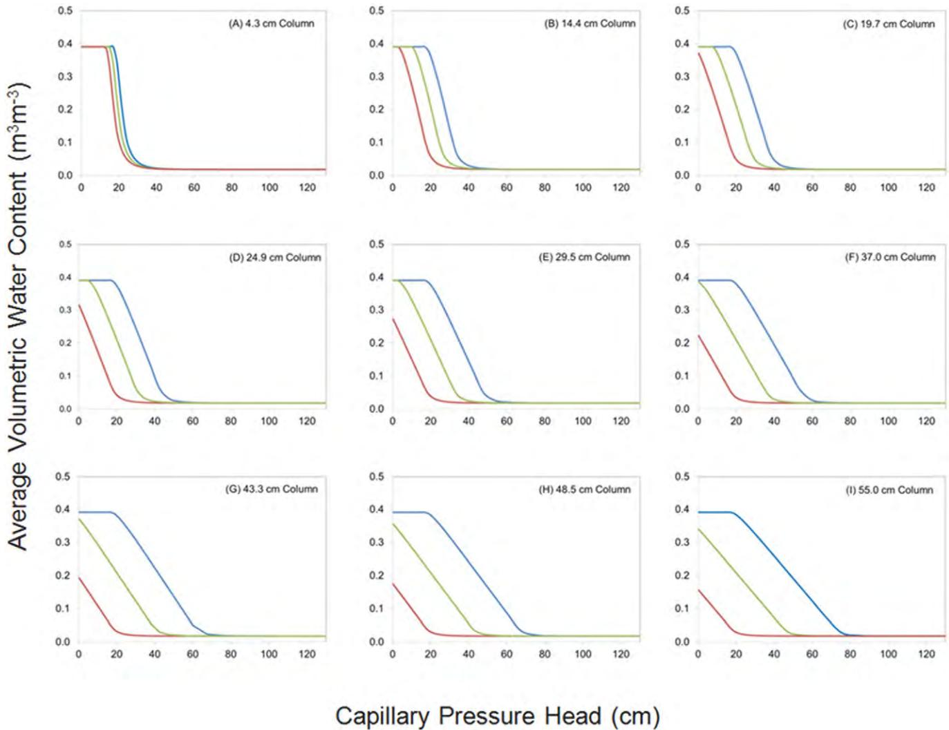
Fig. 3. Comparison of the choice of bottom (red), middle (green), and top (blue) reference pressure elevations in Eq. [2] on predicted average volumetric water content–capillary pressure head functions for nine columns of Flint sand with different heights ranging from (A) 4.3 cm through (I) 55.0 cm.
