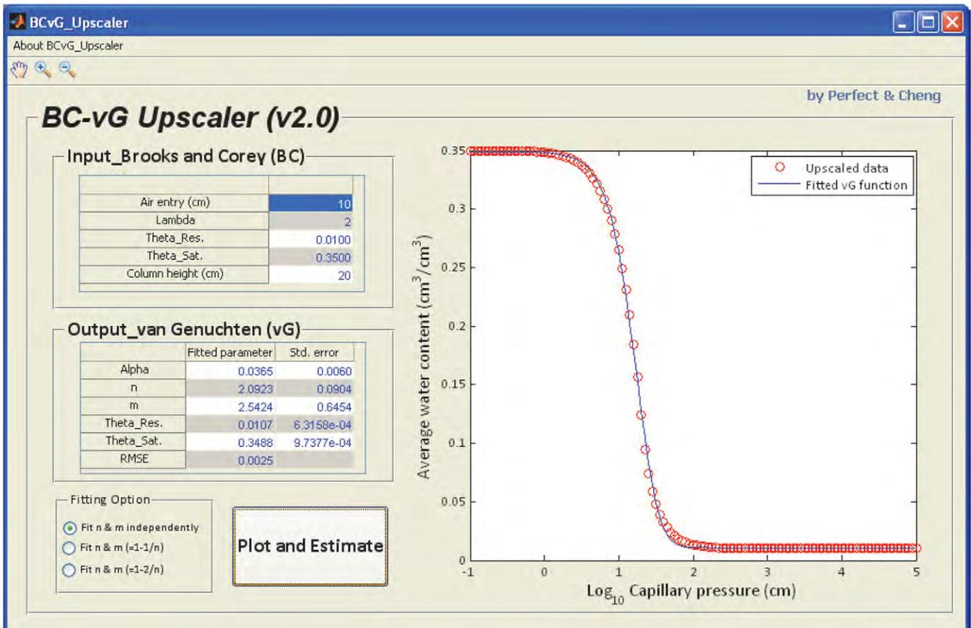
Fig. 2. Screen capture image of the BC-vG Upscaler, showing an example of a height-averaged capillary pressure–saturation function with point Brooks and Corey parameters as the input and average van Genuchten parameters with  $n$  and  $m$  fitted independently as the output for a column height of 20 cm (adapted from Cheng et al., 2013).
