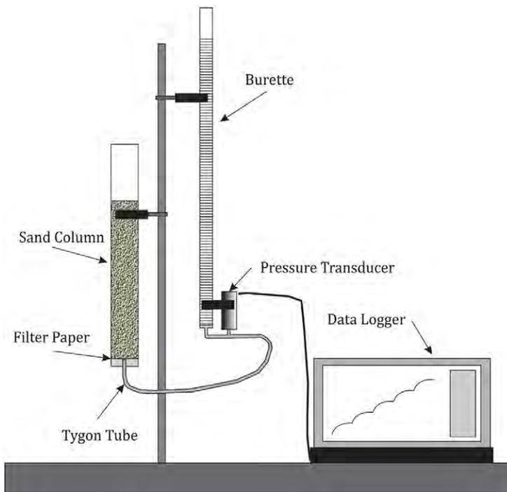
Fig. 1. Hanging water column setup showing sand column, burette, pressure transducer, and data logging computer (adapted from Cropper et al., 2017).
